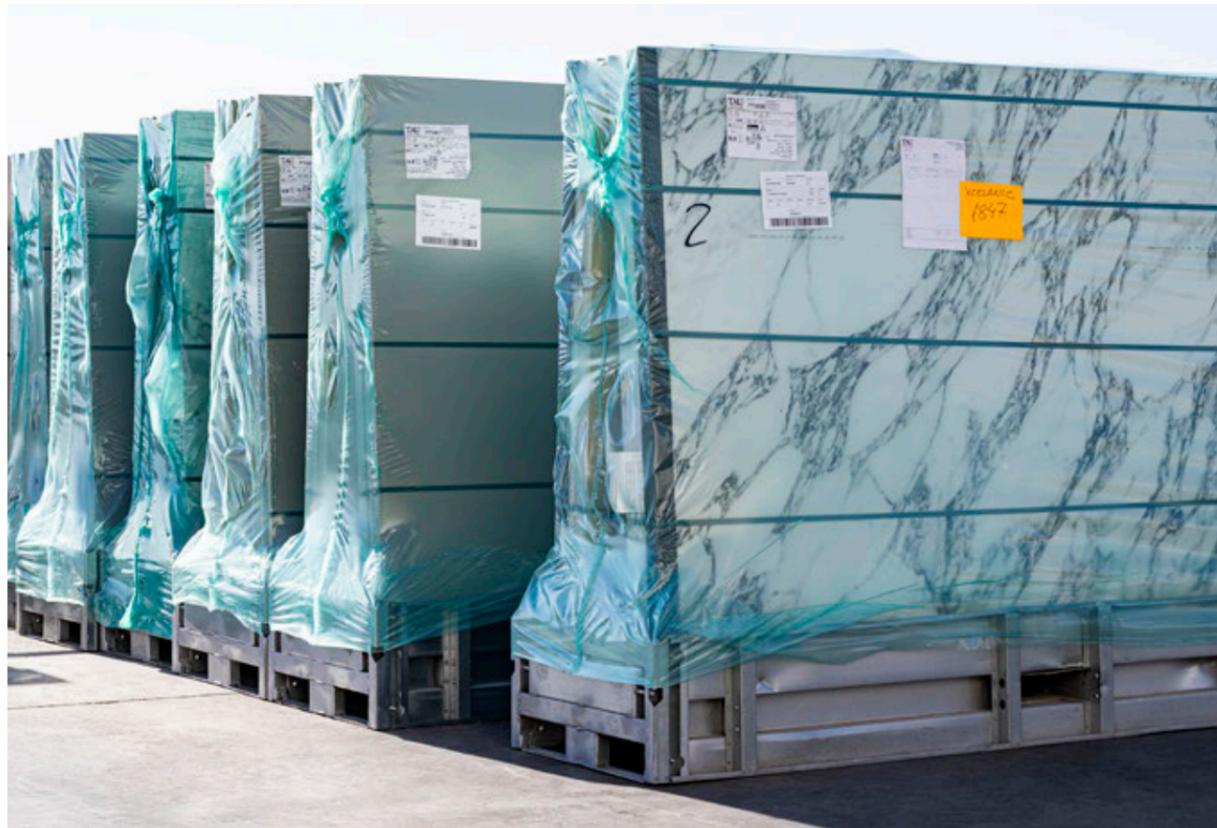
A-Frame with ASCALE slabs must be loaded, unloaded and moved using a proper lift truck, crane or other handling mechanism.
