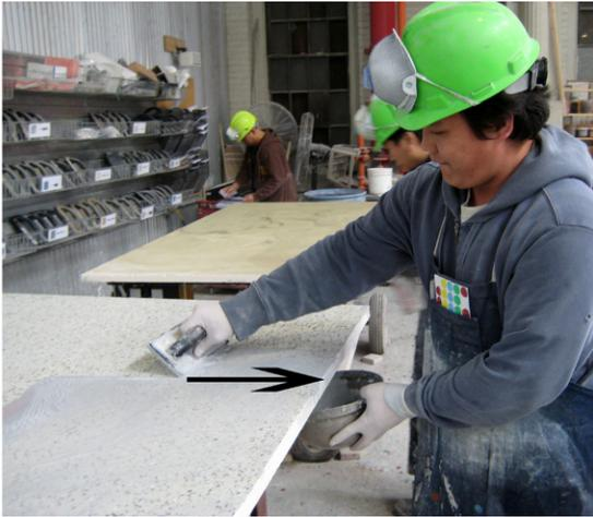
6. Scrape excess slurry into the mixing bowl. Make sure the patch dries in a consistently thin layer. Areas with too much patch will appear discolored and will require reworking.
