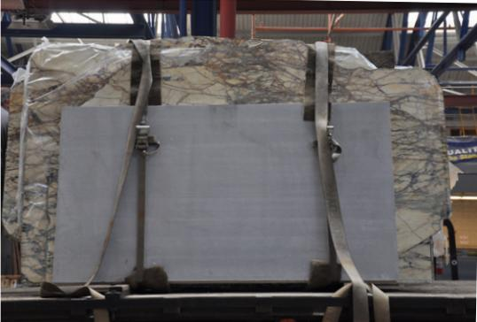
5. This picture illustrates an IceStone slab on a A-frame secured to the truck against a backer slab. Slabs should be loaded face to face, back to back. All loose slabs of IceStone must be loaded on a A-frame that is secured to a truck. While backer slabs are not mandatory, it does offer more protection than a slab being flush against a metal or wooden A-frame.
