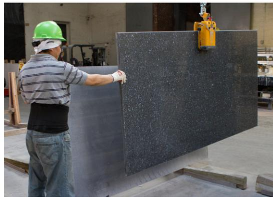
4. Place the first slab on the pipe rack or A-Frame with the polished face against the frame or rack.
