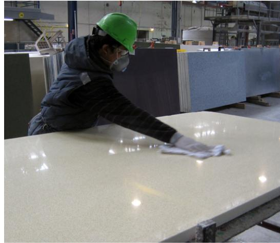
7. Wait until the patch has completely dried. Once dry, wipe off all the dried material from the surface with a clean cotton cloth. The pores should be filled and level.
