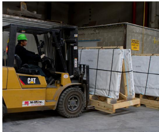
1. Unload delivery crate from the flat bed or LTL box truck using a forklift. Always move crates with a forklift. Do not push, pull or drag crates. IceStone crates are for delivery purpose only. Do not store IceStone slabs on delivery crates.
