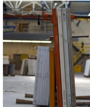
7. When stored on pipe racks, slab should not be vertical; instead, position the slab at an approximately 20 degree angle from vertical position.
