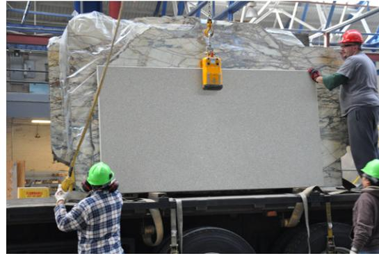
1. At least two people must guide the slab to the designated truck. If the slab is being moved with an overhead crane, one worker should operate the crane, while the other steadies the slab as to reduce extraneous movements which could result in cracking. If the slab is being moved via a boom, one worker should operate the forklift, while the other worker steadies the slab.
